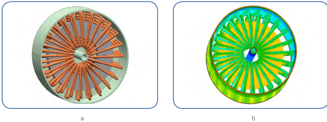
Figure 7. High frequency toroidal core inductor: a) 3D FEA model; b) Temperature field distribution
